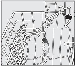
■ Pull the support bar upwards and click it back into position at the required height.
